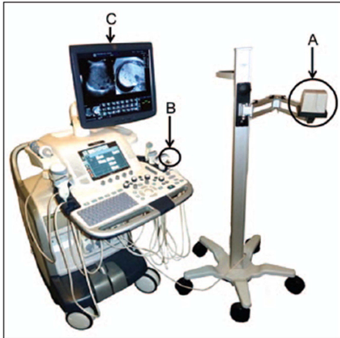
Fig. 2 —Photograph shows fusion imaging system (Logiq E9, GE Healthcare) used for this study. It is composed of position-sensing unit mounted on ultrasound unit (Logiq E9), magnetic field transmitter (A), and two sensors connected to transducer bracket (B). Display of ultrasound unit (C) shows fusion imaging combining conventional sonography and hepatobiliary phase of contrast-enhanced MRI with gadolinium-ethoxybenzyl-diethylenetriamine pentaacetic acid. Used with permission of GE Healthcare
